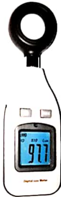
Picture 6 Nishant NE 1010 Lux meter Nishant NE 1010 Lux meter is used to measure the lux levels.
