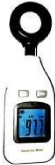
Picture 6 Nishant NE 1010 Lux meter Nishant NE 1010 Lux meter is used to measure the lux levels.
