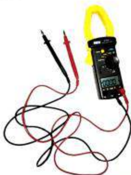
Picture 2 MECD 3159 DIGITAL CLAMP METER
